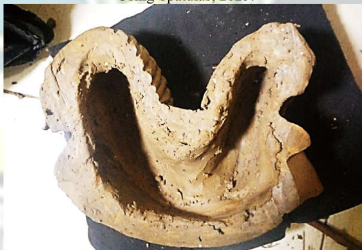
Plate VIII: Sample of Uniform Thickness of Approximately 2cm to Ensure Even Heat Distribution, Bayode Olu-Ojo, 2025.
