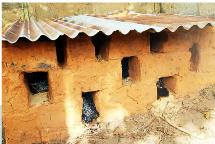
Plate IX: A Locally Constructed Kiln with Red Bricks by the Researcher, Bayode Olu-Ojo, 2025.
