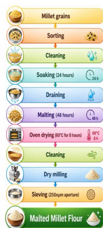
Figure 1. Flow Chart for the Production of Malted Millet Flour ( modified from: Okpalanma et al. (2021))
