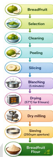
Figure 3. Flow Chart for the Production of Breadfruit Flour (Source: Olaoye, et al (2015))
