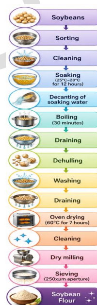
Figure 4. Flow Chart for the Production of Soybean Flour ( modified Iwayemi & Ikujenlola (2025))
