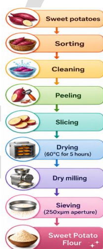
Figure 2. Flow Chart for the Production of Sweet Potato Flour (Modified from Eid et al., (2025))
